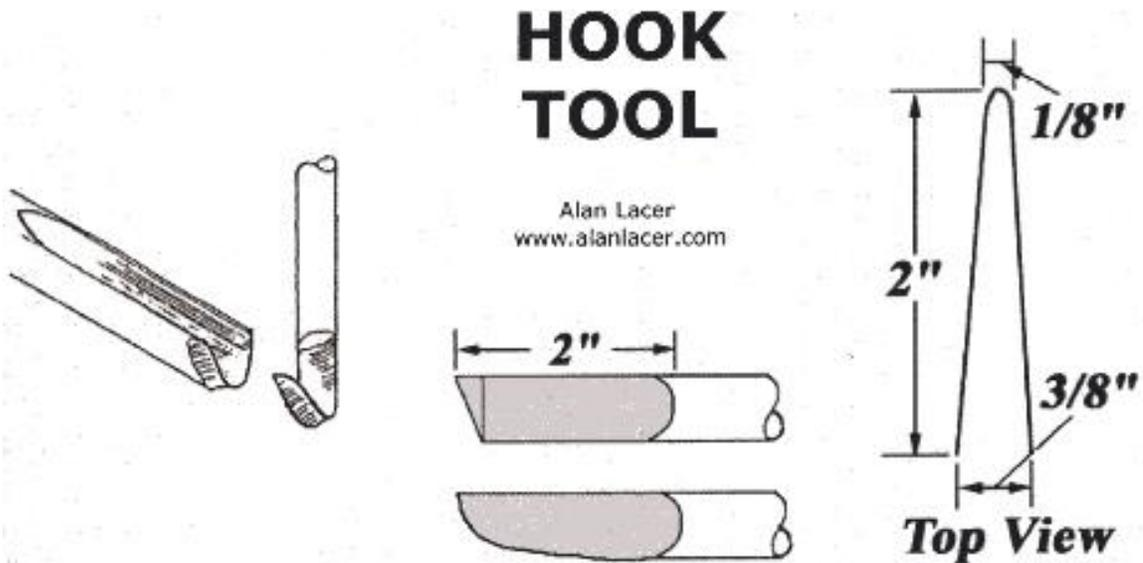
Drill rod of "O 1" tool steel, 3/8" diameter, 9" length, mounted in a handle
