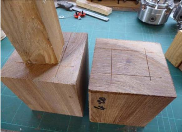
Hot melt glue is normally used to hold scrap wood onto the cube of timber.
