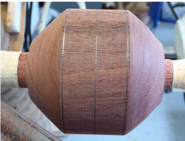
Next we turn a rough shape for the sphere, if you multiply the diameter by 0.297 1.18" (29 mm) and mark a line in from each end and down on each end face we can turn between these lines to remove the waste on each side of the sphere.
