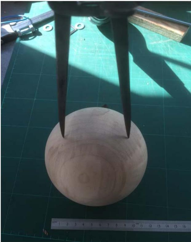
Set a pair of dividers to just over the radius of the sphere 2.2" (55mm) and mark two points on the sphere. Take into account any interesting grain of features.
