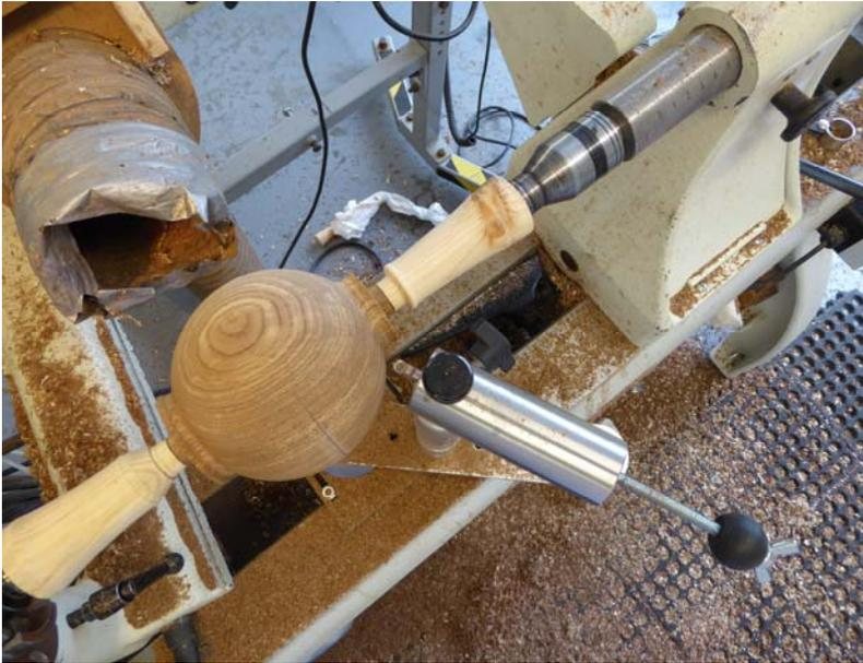
After sanding cut the stubs off with a saw leaving sufficient material to turn the finished sphere.
