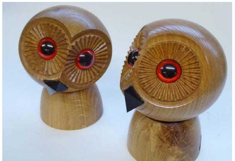
The beak can be made from a piece of Ebony about 0.75" (20mm) Square and sanded to shape. The base is about 2.4" (60mm) dia at the base and tapered up to the top about 2-3" tall with a dish in the top to accept the shape of the sphere.
