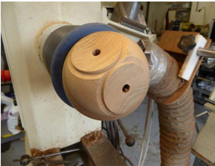
To turn the eyes the sphere can be held in a vacuum chuck or a simple chuck as shown above. Centre the sphere on one of the marks made with the dividers and drill a 0.25" (8mm) hole. Turn the first face as shown in the picture, then rotate the sphere to turn the second face.
