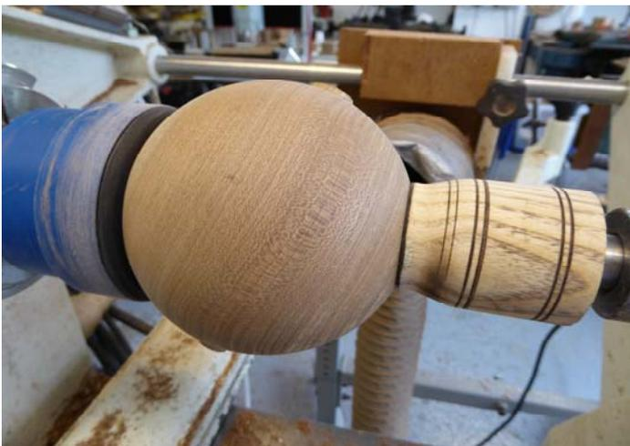
Sphere trapped between cup chucks. I use a bowl gouge to turn off the stubs.
